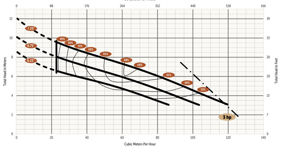
Stated efficiency values are hydraulic efficiency. Wire-to-Water (total) efficiency information is available upon request.
